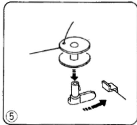
5. Hold the free end of the thread in your hand and press the bobbin winding button located on the front of the machine. Press the bobbin winding button again to stop the bobbin once it has wound several layers and cut off the protruding string. Press again to finish winding the bobbin. The winder will automatically shut off when finished.
