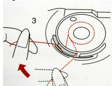
13. Continue to draw the thread lightly until the thread slips into the side notch (B).
