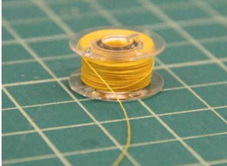
10. Place the bobbin in the bobbin holder with the thread running off counterclockwise.
