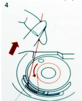
14. Pull out about 4" of thread to the rear. Re-attach the hook cover plate.
