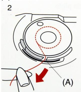
12. Draw thread to the left sliding it between the tension spring blades.
