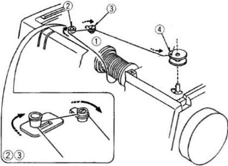
4. Pass the thread through the hole in the bobbin from the inside to the outside. Put the bobbin on the bobbin winder spindle. Push the bobbin to the right to lock the bobbin in place.
